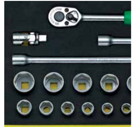
The cut-outs for each tool are created electronically to provide each tool with its own precision milled pocket.
